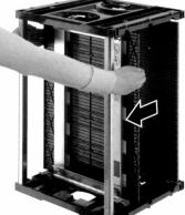
Slide guide rail unit B towards you, then fix the base (top plate) with hexagon socket head cap screws (four
